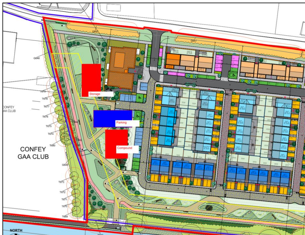
Figure 4: Construction Site Compound
